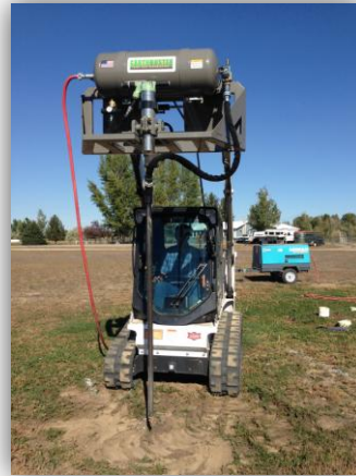
Image 1. EarthBuster device mounted on a skid-steer with air compressor in background.
