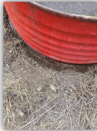
Image 5. Seepage of 1-2" outside the cylinders was not considered significant.
