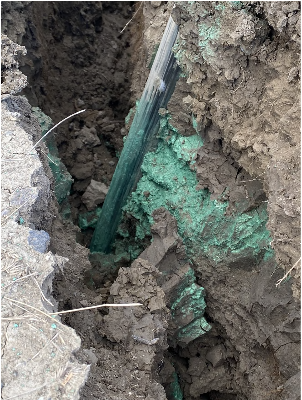
Image C-6: Test #3 - Mica Powder Escaped Between Columnar Peds Towards Surface
