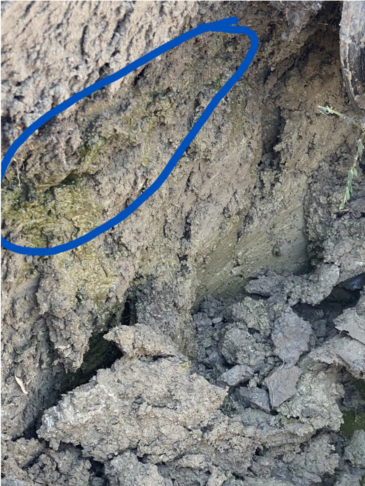
Image C-2: Test 1 - Matcha Green Tea Tracer Powder – Powder absorbed into moist soil
