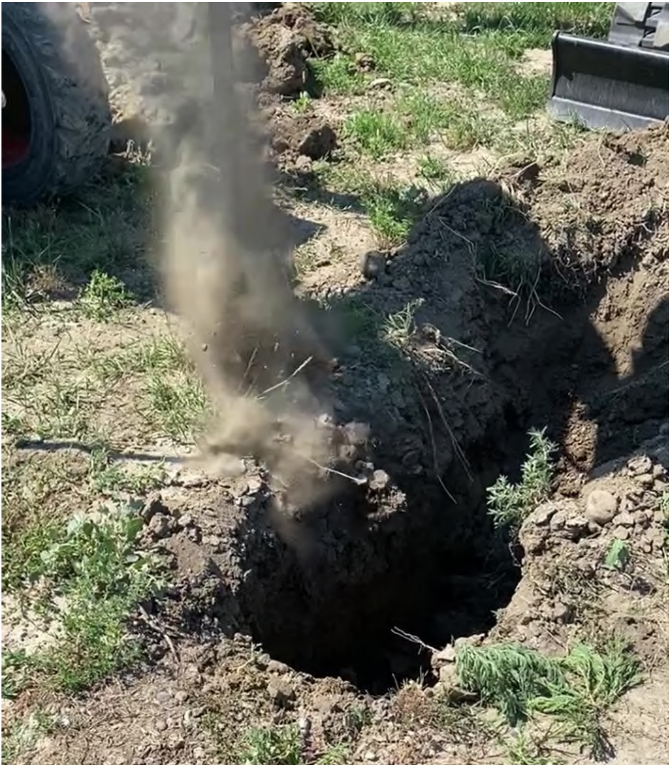
Image C-9: Experimental Test (No Tracer) Air Exiting Vertical Fracture and into Trench
