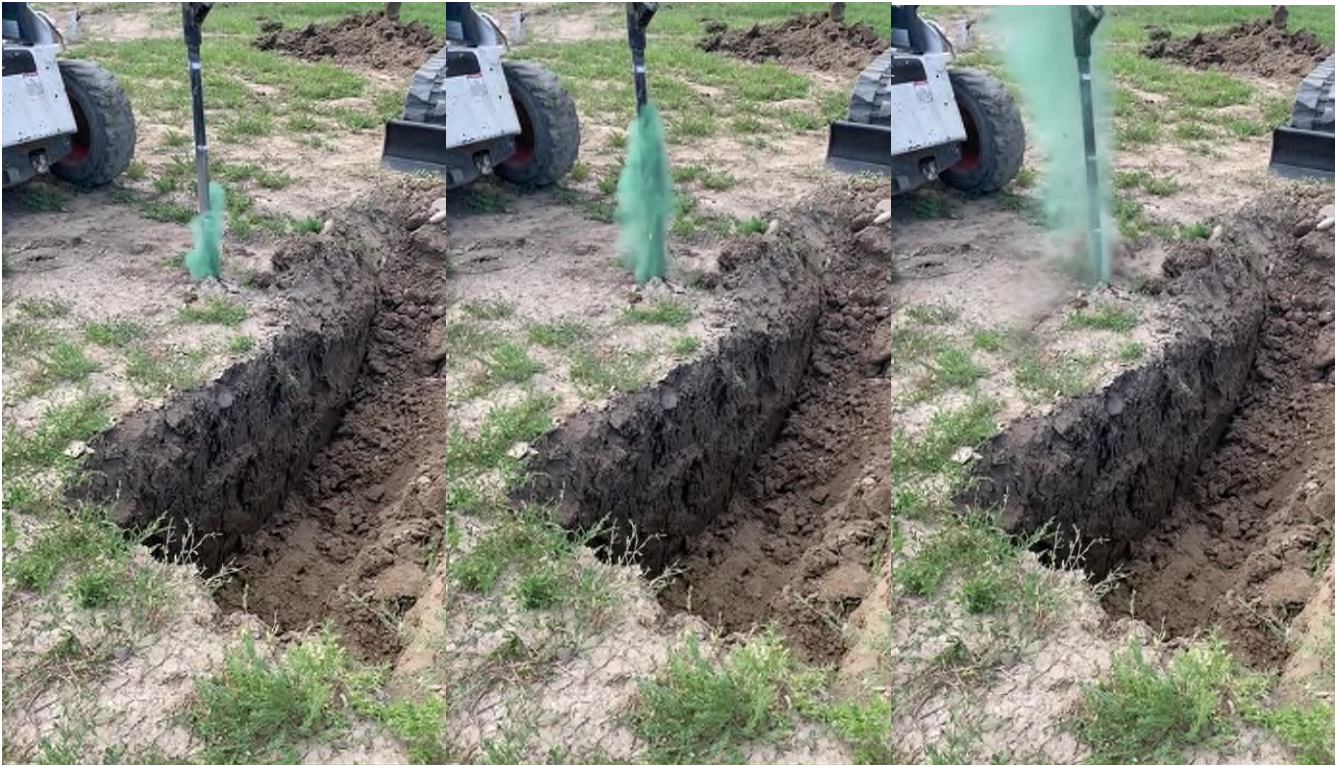
Image C-7: Time Lapse Experimental Test Near Trench (Powder Exiting Near Probe)
