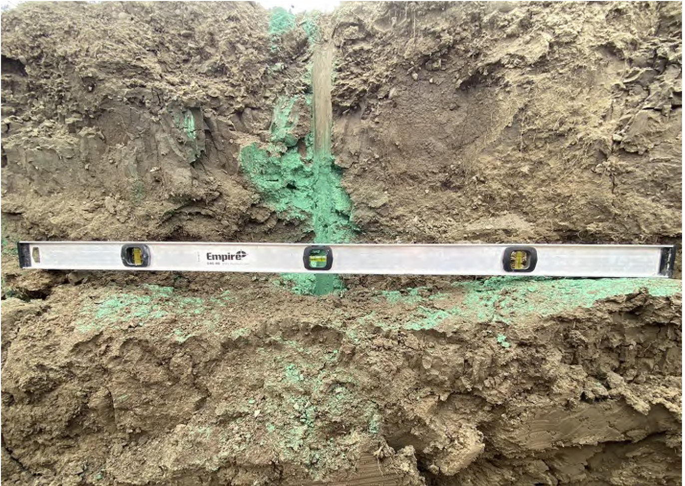
Image C-3: Test #2 - Upward Horizontal Fracture @ 20" Deep with Mica Trace Along Surface of Fracture
