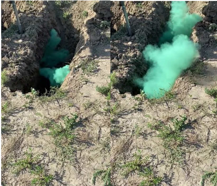
Image C-8: Time Lapse Images - Experimental Test - Mica Powder Exiting into Trench
